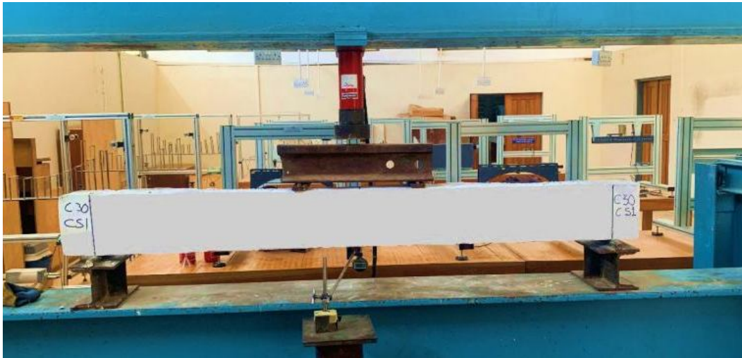
Fig. 2. Beam Testing set-up
