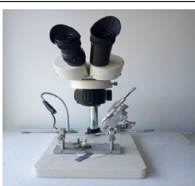
Fig 3: Schely's instrumental insemination device
