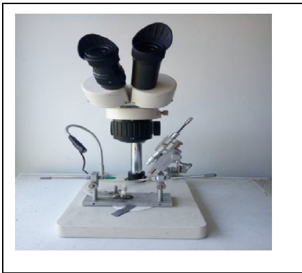
Fig 3: Schely's instrumental insemination device
