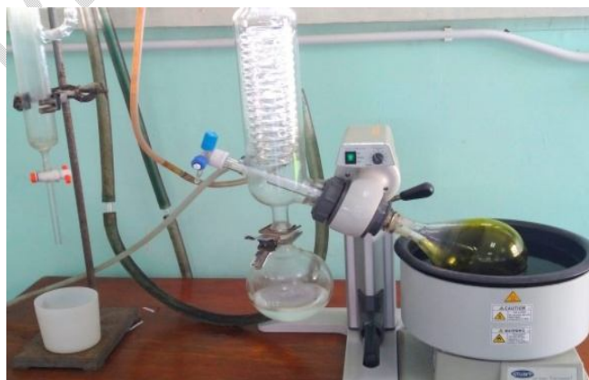
Fig. 2. The rotary evaporator used to concentrate the extracts
