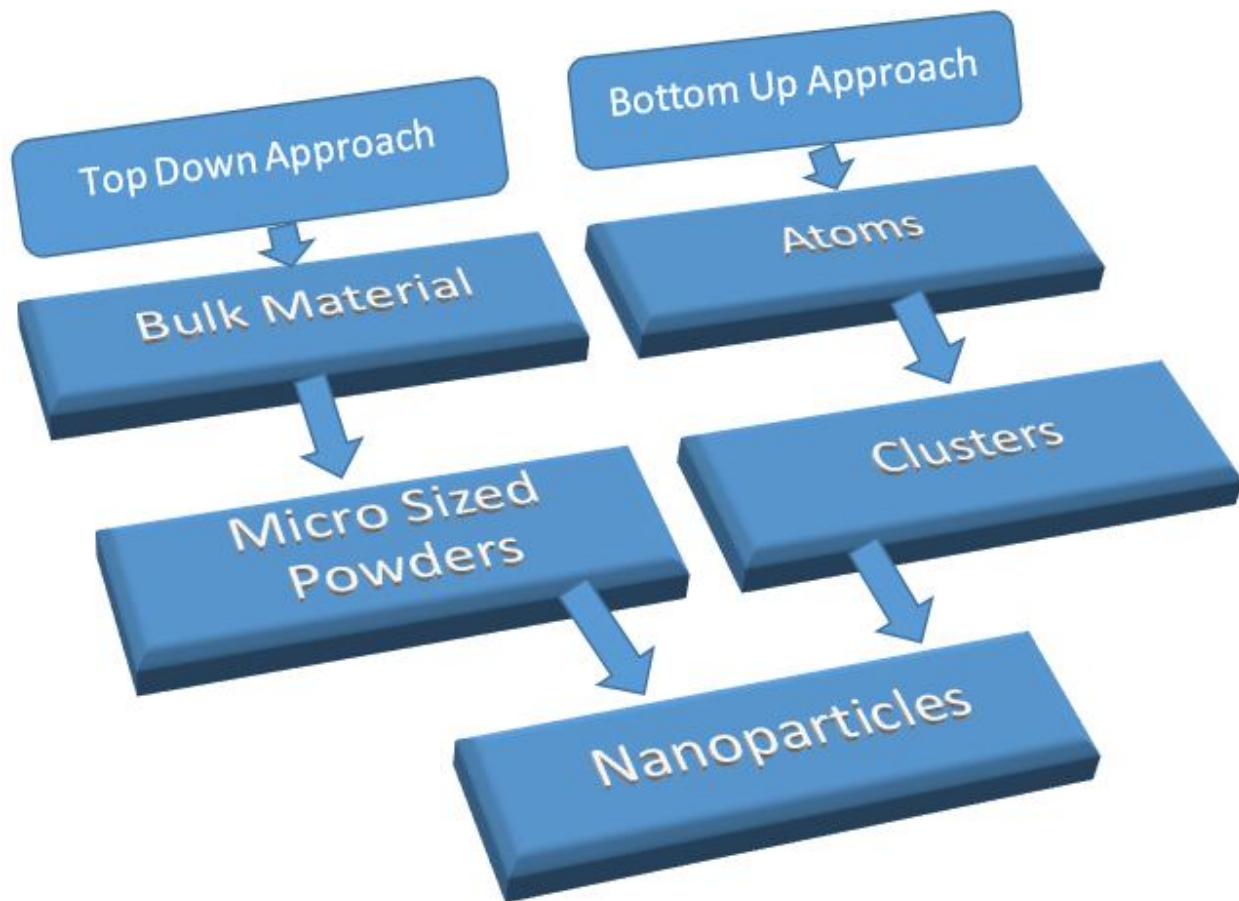
Fig 3 :Nano Fertilizer Synthesis Method
