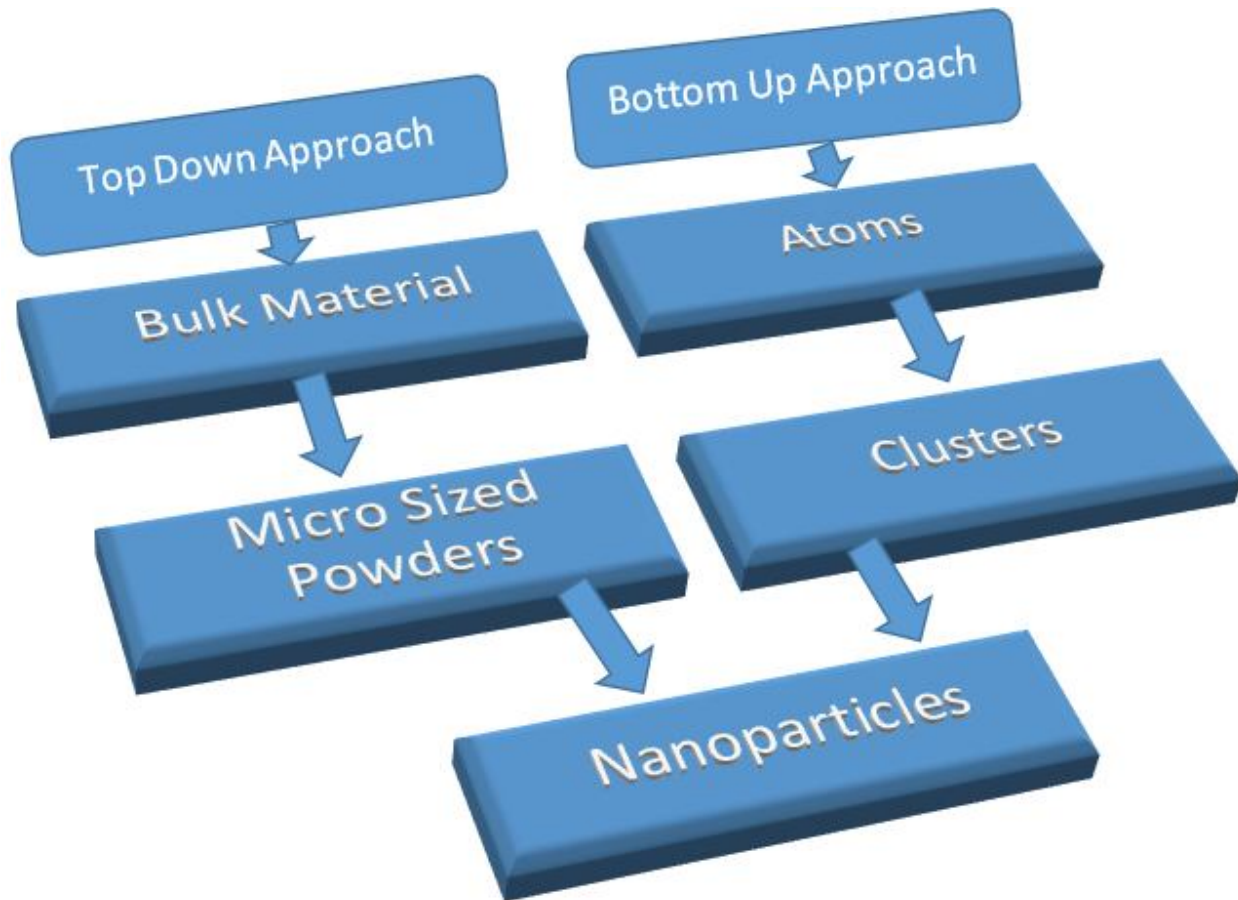
Fig 3 :Nano Fertilizer Synthesis Method
