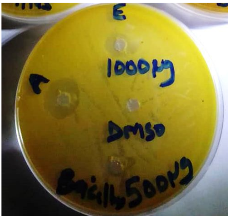
Fig. 9: Fig. 5: Bacterial Activities of the ligand(A) and its Cd(II)(B) against B. subtilis by disc diffusion method
