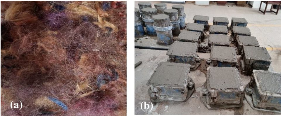
Figure 1: Material preparation: (a) waste synthetic hair fibre, (b) moulding of cube specimens
