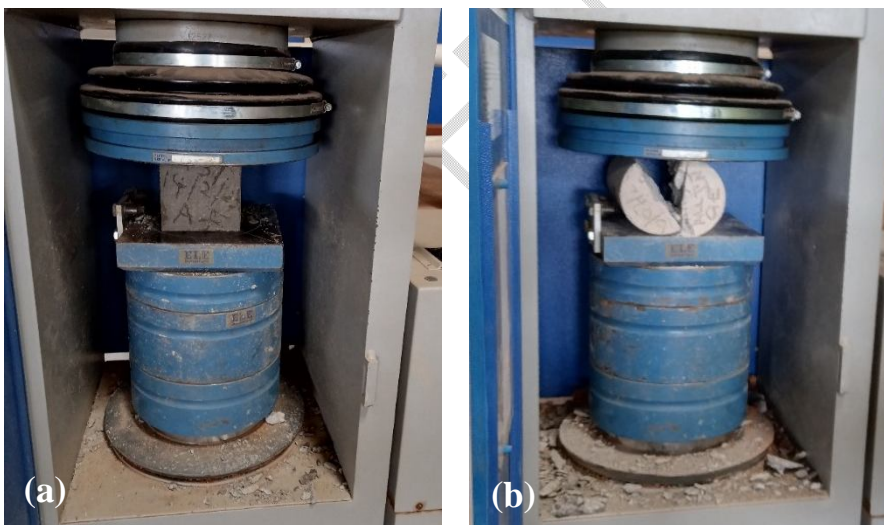
Figure 2: Testing of specimens; (a) compressive strength, (b) tensile strength
