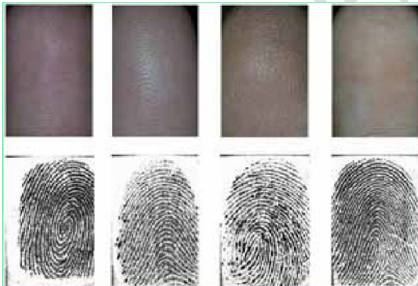
Fig. 4. Database sample images. Top row: touchless finger-prints and bottom row: corresponding touch-based images [12]
