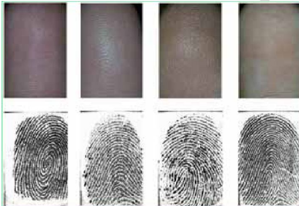
Fig. 4. Database sample images. Top row: touchless finger-prints and bottom row: corresponding touch-based images [12]
