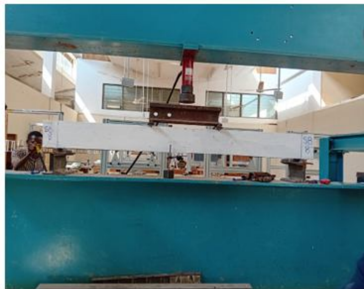
Figure 4: Beam simply supported on a rigid frame
