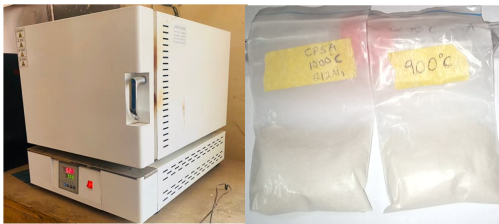
Figure 1: (a) Smokeless Muffle furnace (b) Synthesized CaO biocatalyst in ziploc bags.
