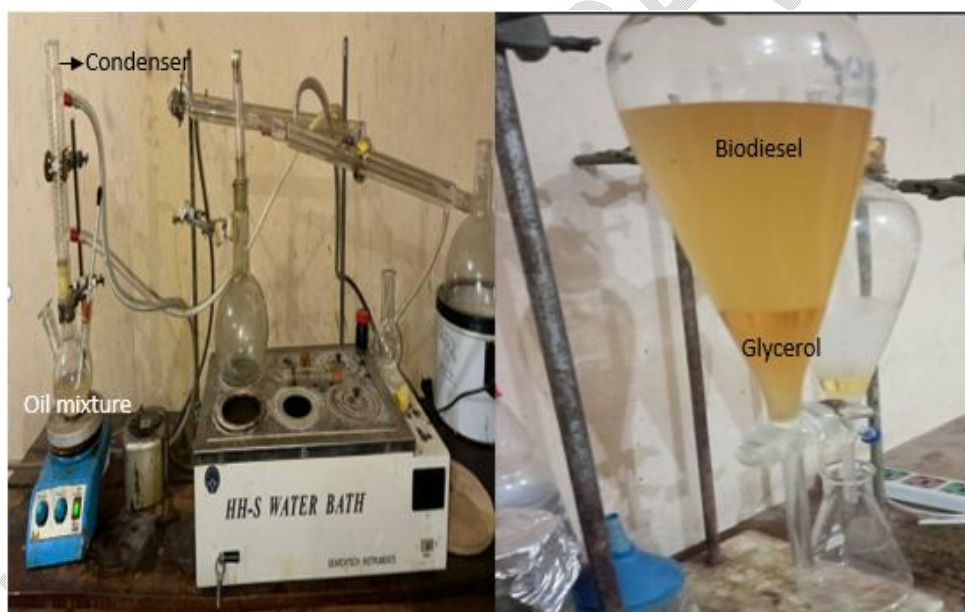
Figure 2. (a) Transesterification set-up, (b) Biodiesel mixture
