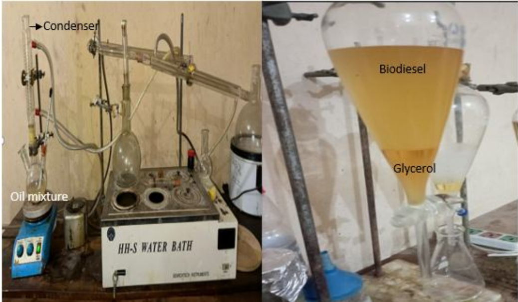
Figure 2. (a) Transesterification set-up, (b) Biodiesel mixture
