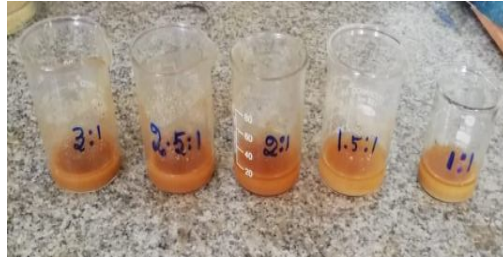
Fig 3. Solubility testing of dried tamarind pellets
