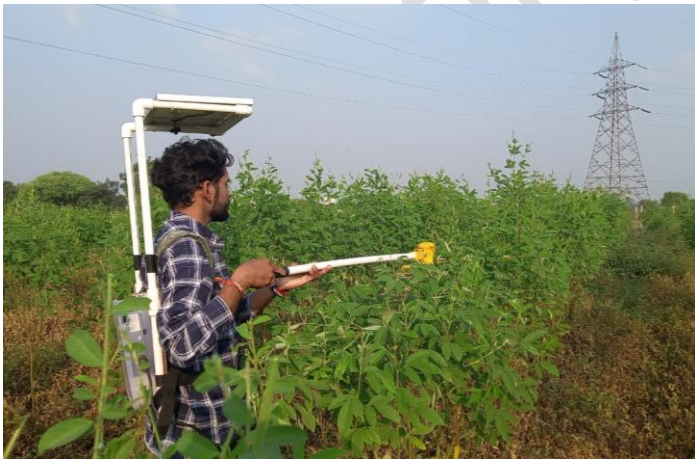
Fig 8. Pruning of pigeon pea by developed pigeon pea pruner
