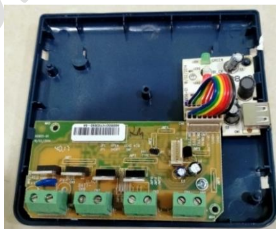
Fig 4. Solar charge controller cicuit board
