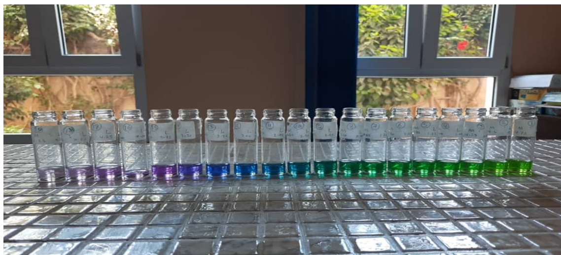
Figure 6b Photo showing colour change after successive addition of ethylene diamine (en) substance to Ni 2+ in ionic liquids (continuous variation method).
