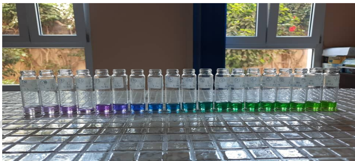
Figure 8b represents photo the colour change after successive addition of ethylene diamine (en) substance to Ni 2+ in ionic liquids (continuous variation method).
