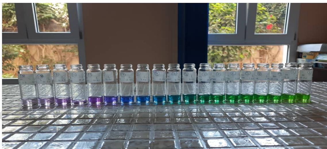
Figure 8b represents photo the colour change after successive addition of ethylene diamine (en) substance to Ni 2+ in ionic liquids (continuous variation method).
