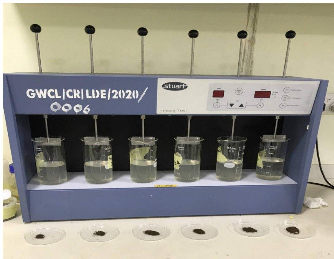
Figure 6: Flocculation of Water Samples with Prepared Coagulants using SW6 Stuart Rotor Flocculator at the Ghana Water Company Limited (GWCL) Laboratory
