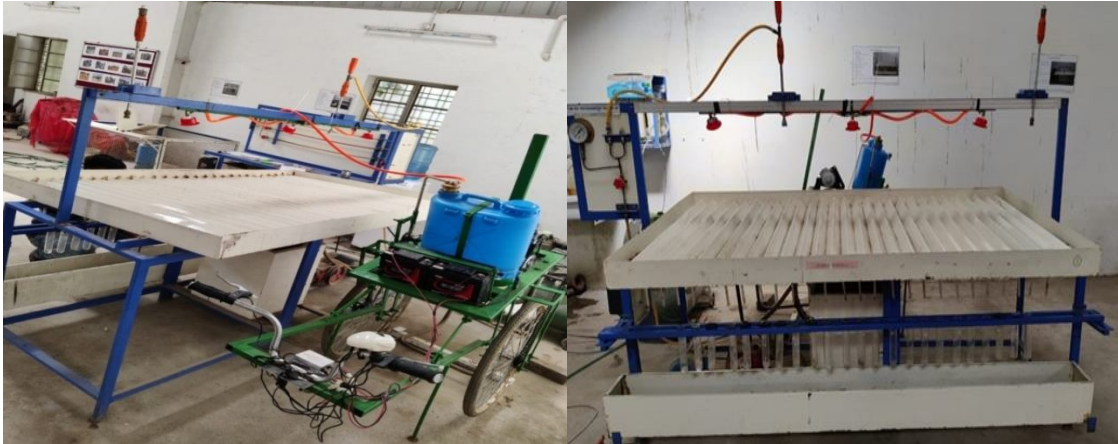
Fig.3 Experiment setup Sprayer patternator setup
