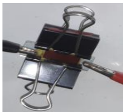
Figure 4: Assembled dye cell
