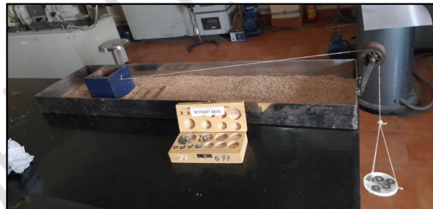
Fig. 2 Measurement of frictional properties of foxtail millet seeds
