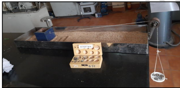
Fig. 2 Measurement of frictional properties of foxtail millet seeds
