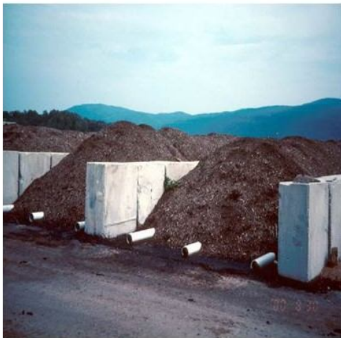
Fig. 5. Passive Aerated Windrow method of composting
