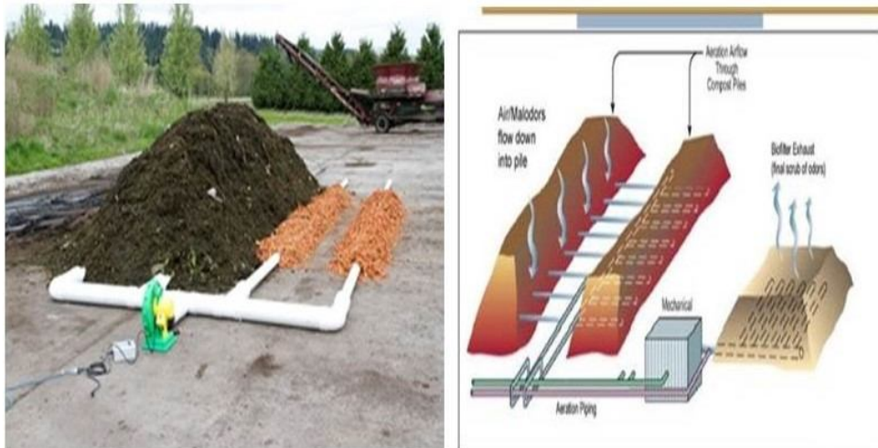
Fig. 7. Aerated static pile method of composting
