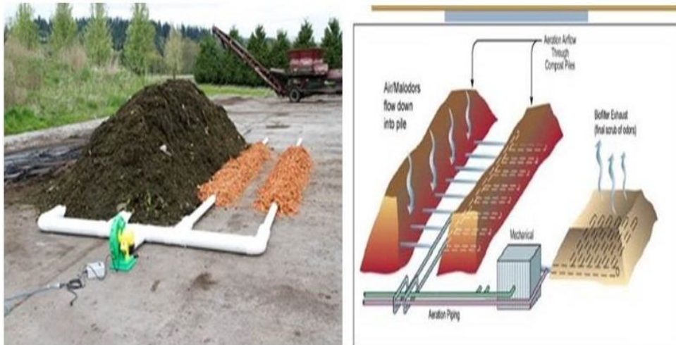
Fig. 2.7. Aerated static pile method of composting
