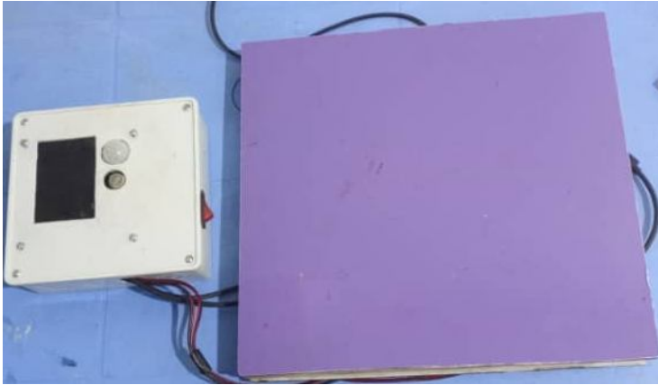
Figure 8: Hardware of the Gas Gauging System
