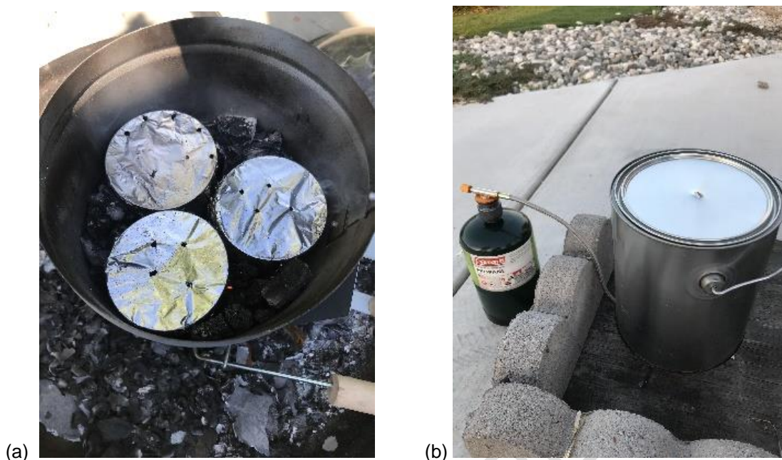
Figure 1. Photographs showing the carbonization setup: (a) chimney starter configuration, (b) gas burner configuration.
