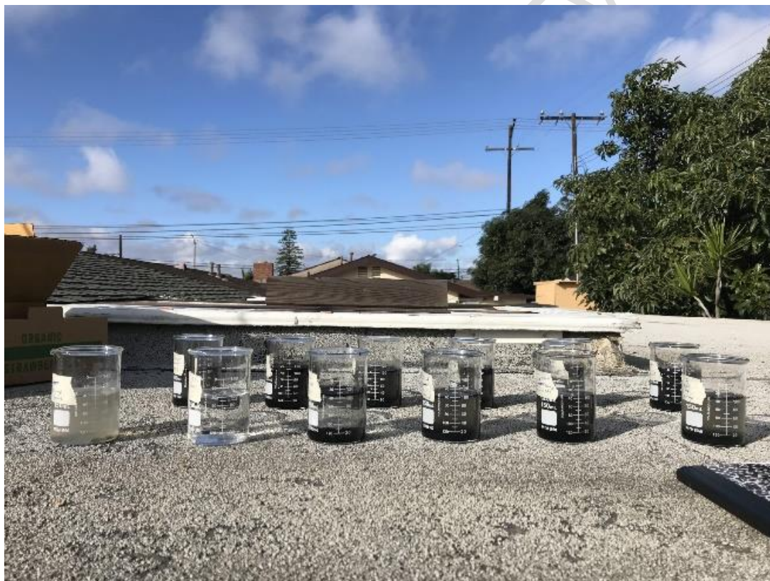
Figure 2. Test setup for solar thermal evaporation experiment.
