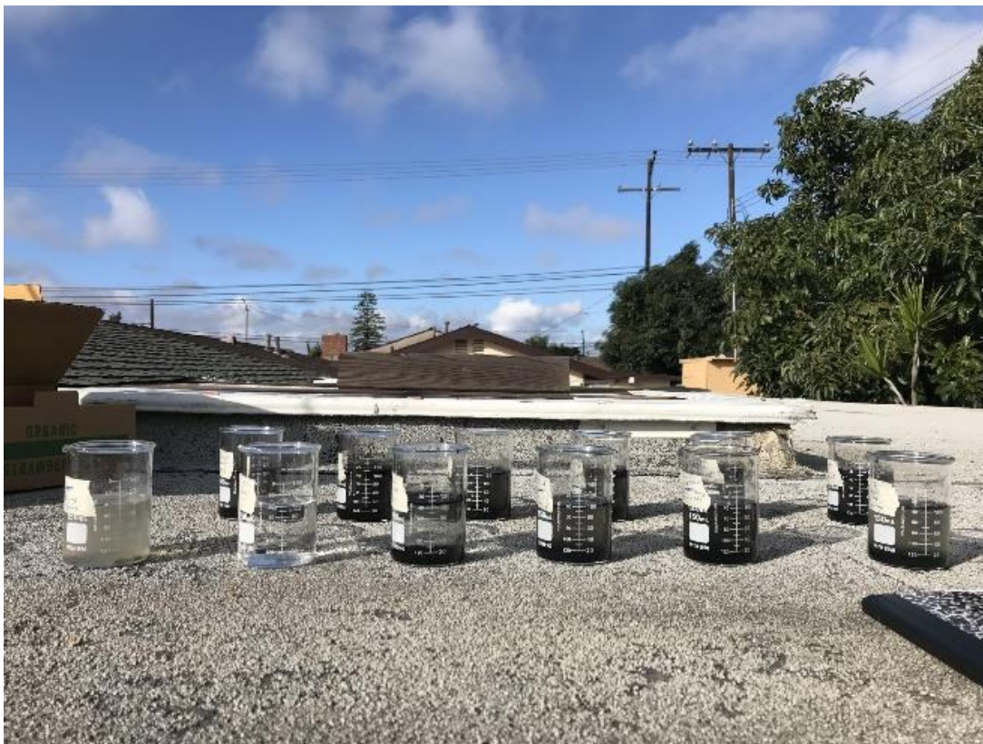
Figure 2. Test setup for solar thermal evaporation experiment.
