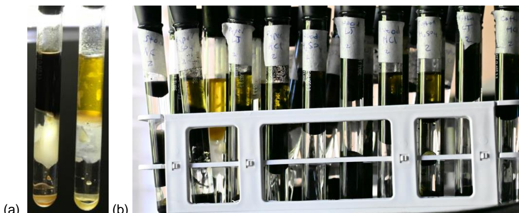
Figure 9. (a) Control samples of 5 mL of used motor oil and olive oil and (b) AC samples in olive oil after testing for 2 weeks. Case A 10 can be seen on the far left for the commercially available activated carbon (CAC).
