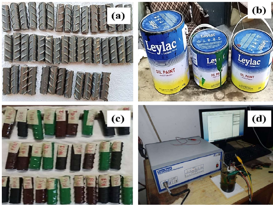
Fig. 3: a- Rebar before, b – Selected paints, c – Rebar after coat, d - Model CS350 station setup
