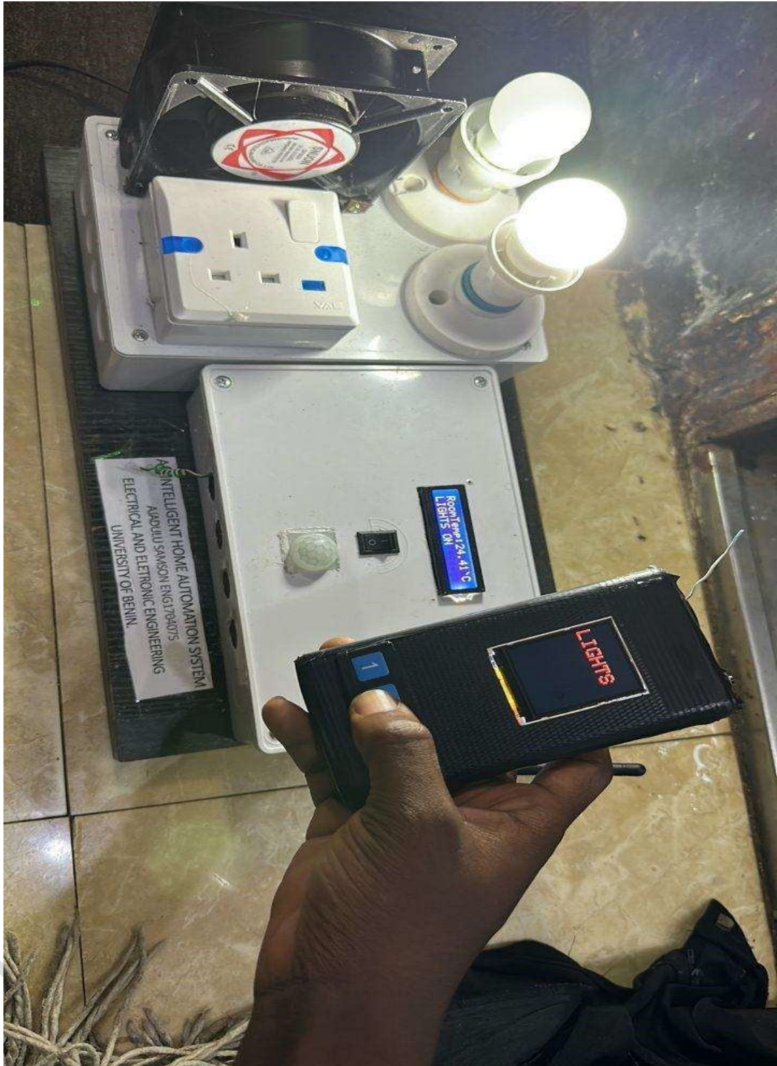
Figure 16. Automated Smart System (When Device is Turned On)
