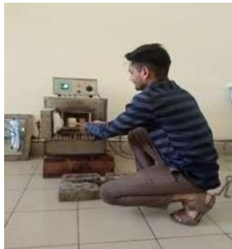
Fig. 5 Muffle furnace for volatile matter and ash content
