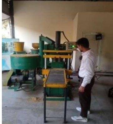
Fig. 2 The biofuel briquettes preparation in briquetting machine
