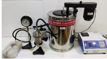
Fig. 4 Bomb Calorimeter for Calorific value
