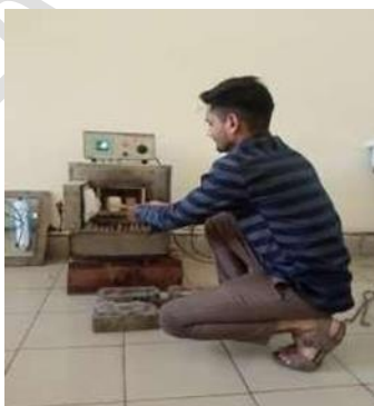
Fig. 5 Muffle furnace for volatile matter and ash content
