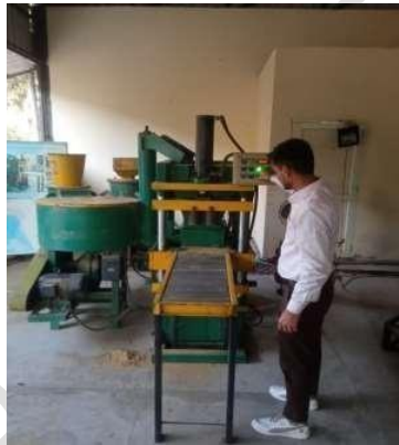
Fig. 2 The biofuel briquettes preparation in briquetting machine
