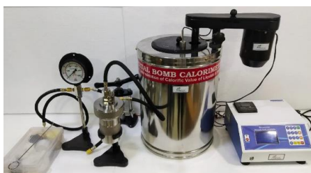
Fig. 4 Bomb Calorimeter for Calorific value
