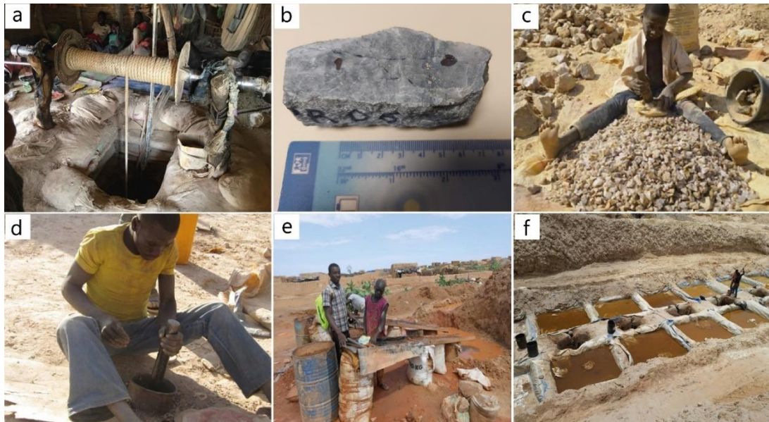
Fig. 3. Stages of artisanal gold mining at Koma Bangou. a) Ore extraction shaft fitted with winch; b) Gold-bearing quartz; c) Manual ore crushing; d) Manual ore grinding; e) Gravity gold concentration with sluice; f) Cyanide leach tanks.
