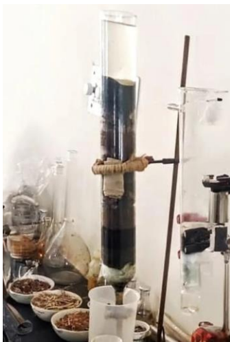
Image 1 Filter Column set up for Sawdust
