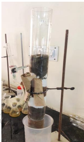
Image 2 Filter Column set up for Limestone
