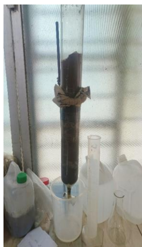
Image 4 Filter Column set up for Vetiver
