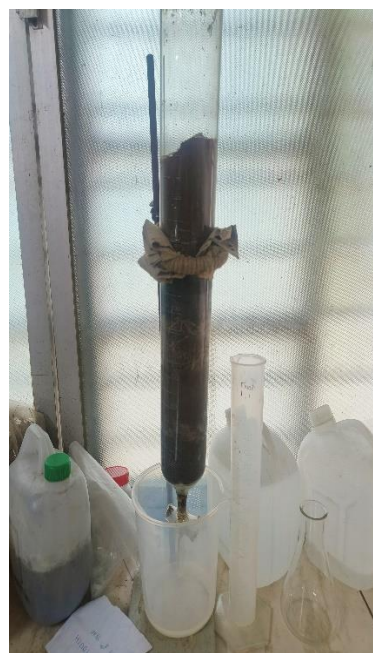
Image 4 Filter Column set up for Vetiver
