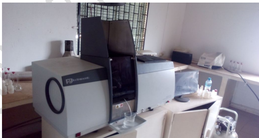
Figure 6: Atomic absorption spectroscopy (AAS) setup
