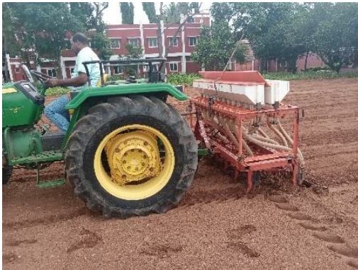
Plate 2. Tractor operated seed cum fertilizer seed drill in the actual field
