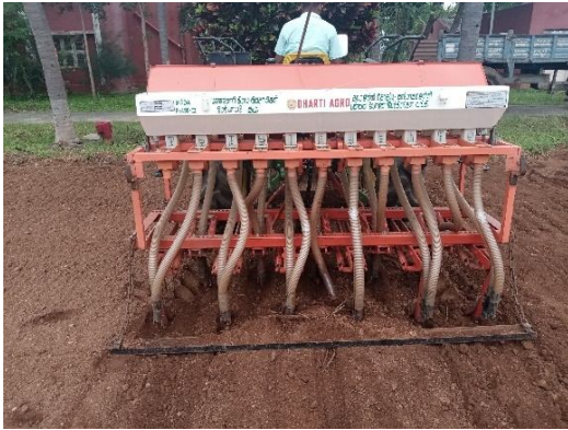
Plate 1. Tractor operated seed cum fertilizer seed drill for sowing ragi seeds
