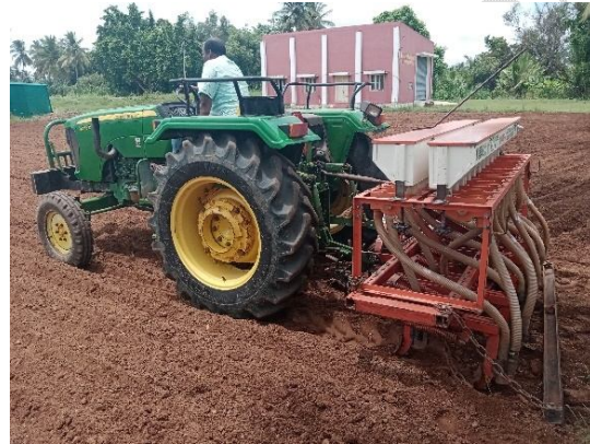
Plate 1. Tractor operated seed cum fertilizer seed drill for sowing ragi seeds
