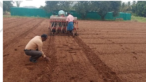
Plate 1. Tractor operated seed cum fertilizer seed drill for sowing ragi seeds
