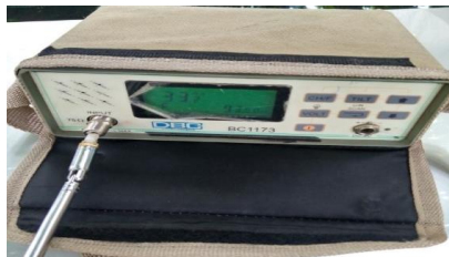
Fig. 1: High Resistance/Low Conductance Field Strength Meter
