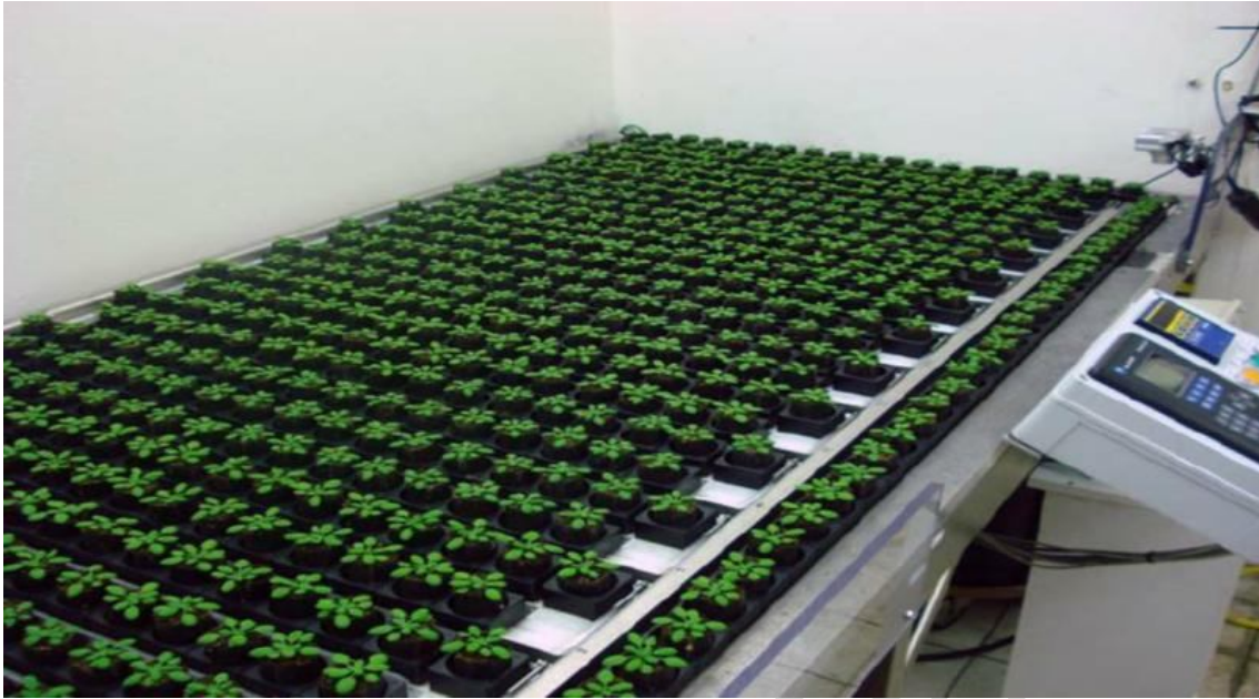
Fig 3 :Phenoscope: Developed at INRA-IJPB Versailles, this Arabidopsis culture system has the ability to grow and move 735 plants across the culture table, individually modify each plant's water and nutrition status, and track each plant's development using picture analysis [27].
