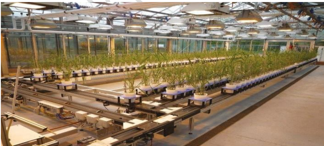
Fig 8 : the LemnaTec platform used in [18] equipped with conveyors to move the plants in acquisition booths
