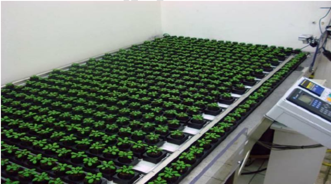
Fig 3 :Phenoscope: Developed at INRA-IJPB Versailles, this Arabidopsis culture system has the ability to grow and move 735 plants across the culture table, individually modify each
