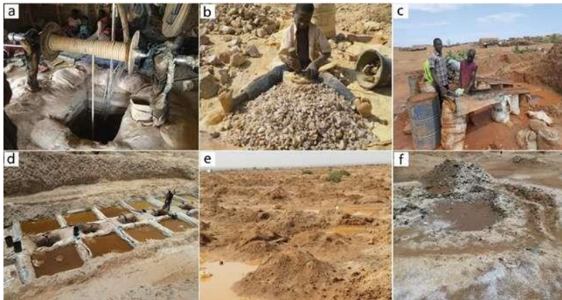
Fig. 2. Stages of artisanal gold mining at Koma Bangou. a) Ore extraction shaft fitted with winch; b) Manual crushing of ore; c) Gravity concentration of gold in sluice; d) Cyanide leach tanks for gold-bearing ore; e) Spreading of cyanidation waste; f) Acidification waste dump.
