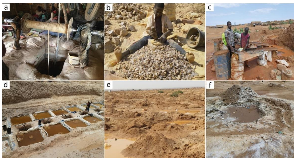
Fig. 2. Stages of artisanal gold mining at Koma Bangou. a) Ore extraction shaft fitted with winch; b) Manual crushing of ore; c) Gravity concentration of gold in sluice; d) Cyanide leach tanks for gold-bearing ore; e) Spreading of cyanidation waste; f) Acidification waste dump.
