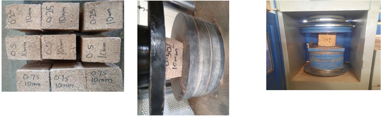
Figure 3: specimen and testing, (a) specimen, (b) compressive strength test, (c) tensile strength test
