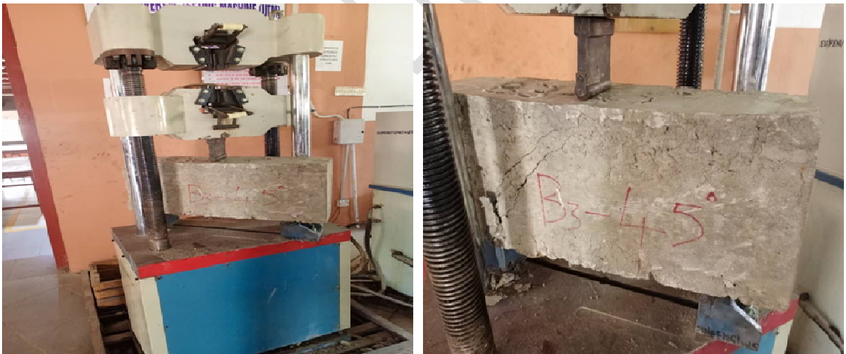
Plate 1: Loading of beams with 90° and 45.0° shear reinforcements
