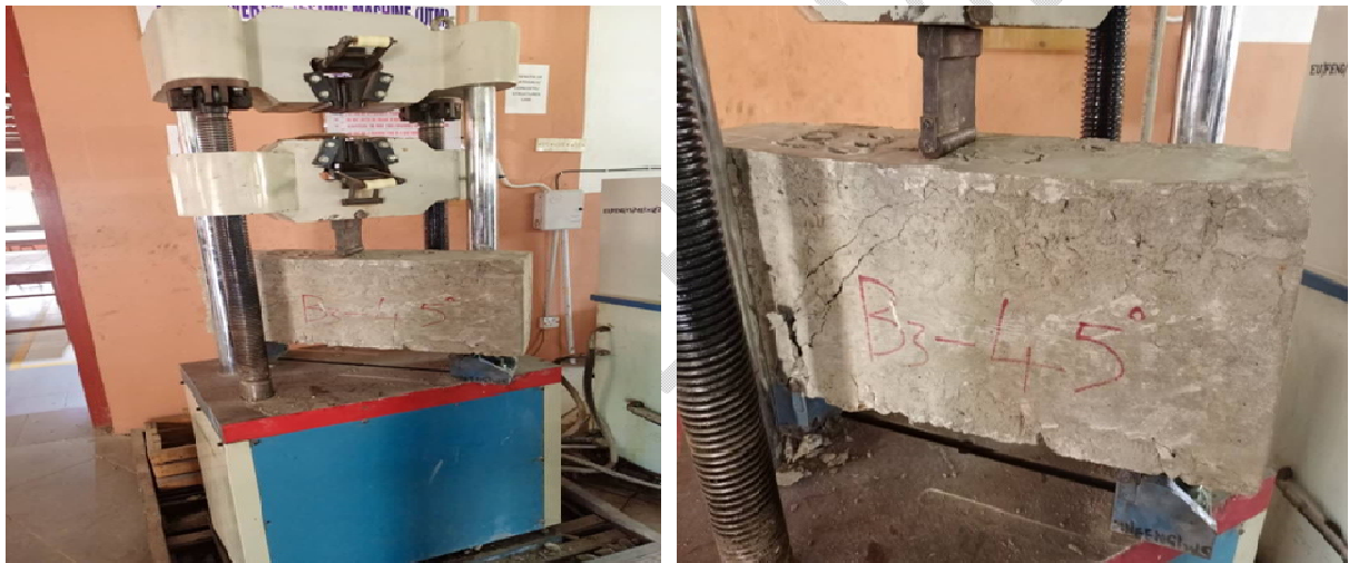
Plate 1: Loading of beams with 90 0 and 45.0 0 shear reinforcements
