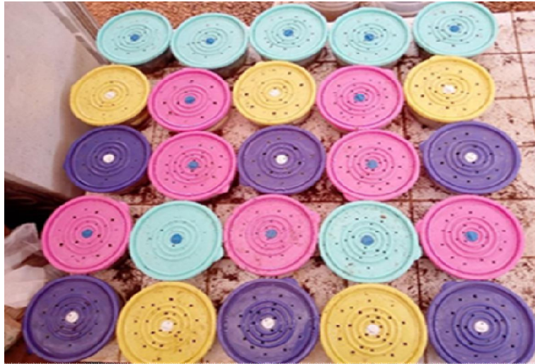
Fig4: Composter made of 1.5 L plastic boxes
