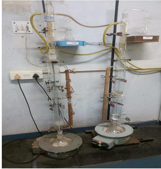
Fig:-1 1Perforator equipment setup used in EN 120 method
