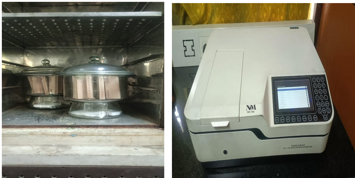
Figure. 2 Apparatus of desiccator set up testing, according to JIS A 1460
