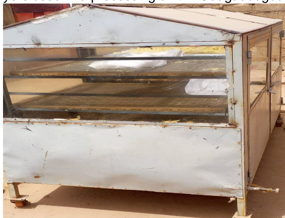
a. Hybrid dryer (solar and gas)
